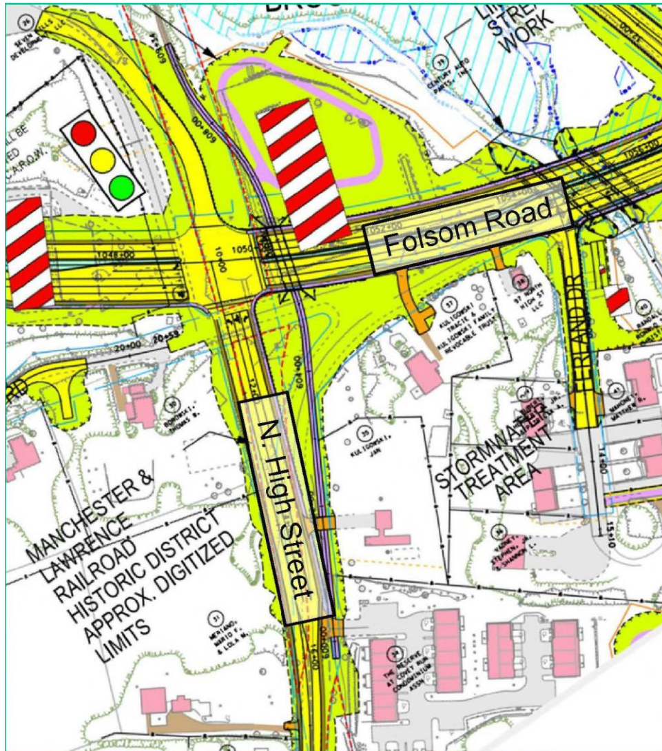
Exhibit 1: Underpass Alternative design showing the tunnel beneath Folsom Road and route of the proposed 900-foot path. Admin. Rec. at 0009708.
